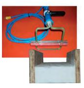
= Panel puller With panels weighing 800 pounds, the panel puller is helpful to slide large panels together on base plates or slide up roof panels into exact position. Regular SIP builders find this tool a must.
