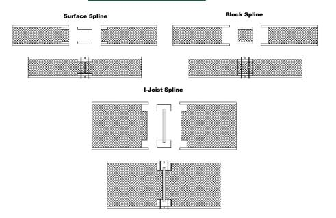
FIGURE 1—SIP SPLINE TYPES
