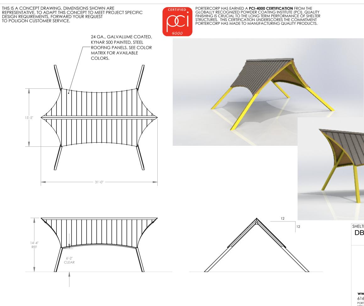
GENERAL FRAME NOTES: 1. ALL STEEL COMPONENTS (STRUCTURAL MEMBERS, ORNAMENTATION, RAILING, ETC.) ARE POWDER COATED IN THE FOLLOWING MANNER (UNLESS REQUESTED OTHERWISE): SHOT BLASTED TO NEAR WHITE • CONDITION (SSPC SP-10) WASHED AND SEALED IN A PHOSPHATE SPRAY PRIME-COATED WITH POLI-5000 HIGH ٠ PERFORMANCE POWDER APPLIED EPOXY TOP-COATED WITH SUPER-DURABLE TGIC POLYESTER POWDER AND OVEN CURED • SEE POLIGON.COM FOR COLOR OPTIONS 2.
