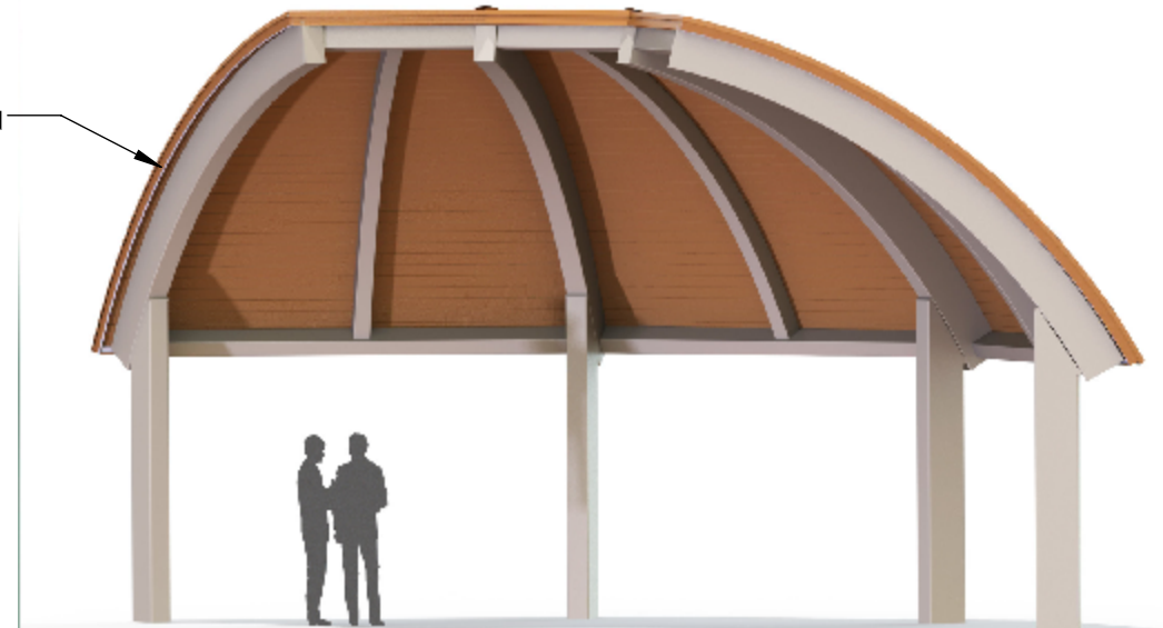
MEGA-RIB METAL ROOFING OVER T&G DECK SHOWN
