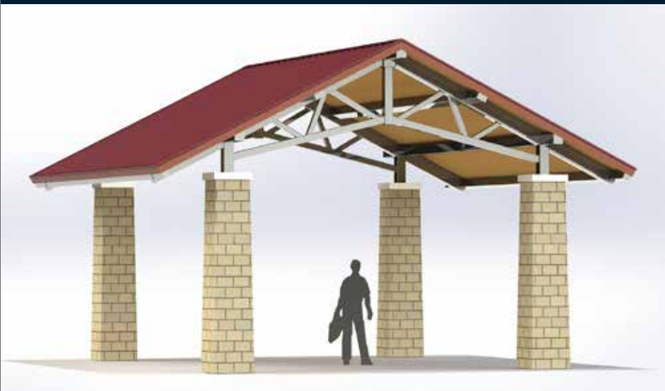
Simple variations can create dramatic results. Here a basic 24 x 24 shelter is given increased overhang, decorative truss treatment, and site-built column wraps. [DB-29]
