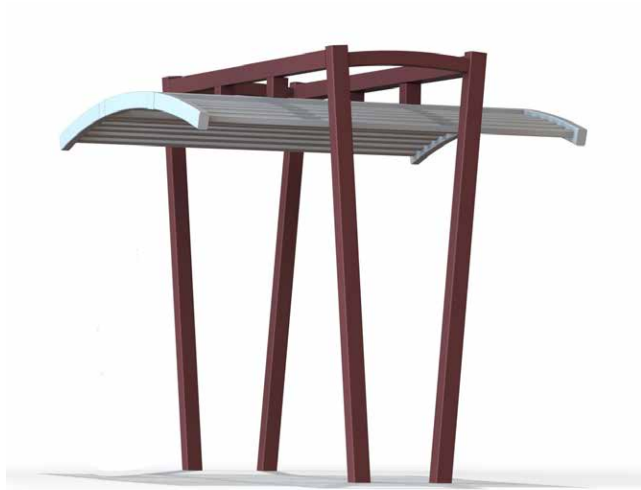
Here is a 11 x 10 arc form trellis supported by a unique diverging column and truss arrangement. This trellis, or a suitably sized variation, could be an entry feature for many buildings. [DB-69]
