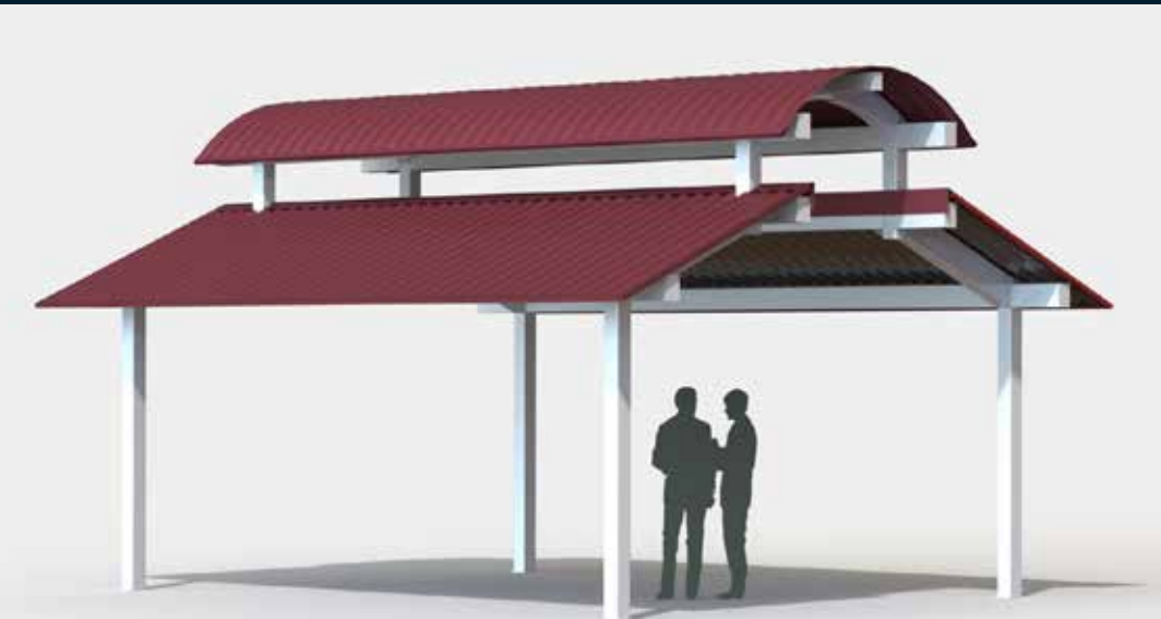
This 20 x 24 shelter sports a combination of a straight, lower roof with an arched upper tier roof. The result is an unusual and distinctive shelter. [DB-19]
