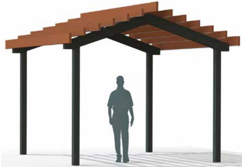
An unusual trellis on which latilla, mounted flat side perpendicular to the ground, ascend the truss framing. This trellis is 12 x 15 in size and latilla can be either steel tube or 4"x8" cedar wood. [DB-65]
