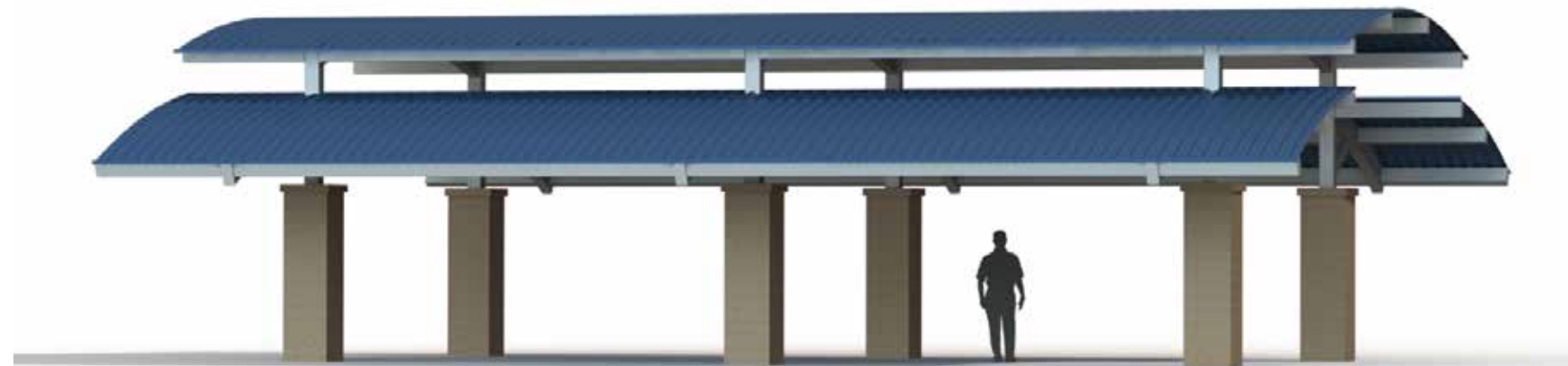
This dramatic 40x52 shelter uses arched roof elements and long cantilevers as key features. [DB-39]
