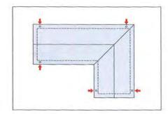
L Shaped Shelters Install downspouts as shown. Add downspouts\* when the distance between downspouts exceeds 24'.
