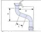
Check the measurement to get the length of the bridge pipe. Use table on right.
