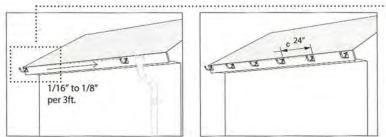
Fasten "high hanger" at the opposite end of roof base. To the slope to the pipes should be 1/16" to 1/8" per 3ft.
