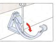
Use screwdriver to fold the tab forward for low angles and back for angles greater than 22°
