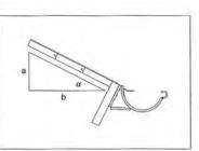
Calculate your roof pitch and adjust the hanger accordingly. See roof layout pages for building pitch.
