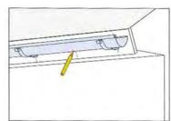
Place the gutter in the hangers and mark out for the plug-in outlet on the gutter.
