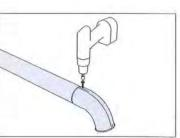
Attach the ground level beaded elbow using self tapping screw on back side.
