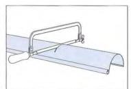
Use a hack saw to cut the gutter.
