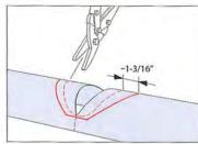
Finish by cutting up to the bead and backside as shown in the picture.
