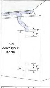
Install two downspout brackets. Add additional brackets if downspout length exceeds 10'.
