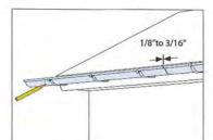
Place the gutter to be joined in the hangers and mark out correct length.
