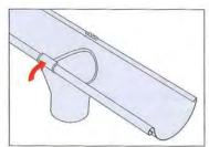
The plug-in outlet snaps easily on the gutter.
