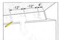
Mark out for the hangers around the downspout.
